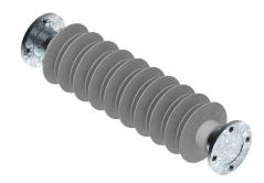
The GRP rod of the RPS insulators is sheathed in highquality grey silicone. The fittings are made of galvanised steel. All composite insulators are design- tested and type-tested in line with DIN EN 62621.
